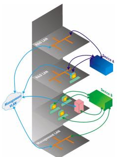
In virtual topological networks, the network devices may be located in diverse places around the LAN—such as in different departments, on different floors or in different buildings. Connections are made through software. Each network device is connected to a hub, and the network manager uses management software to assign each device to a virtual topological network. Elements can be combined into a VLAN even if they are connected to different devices.
